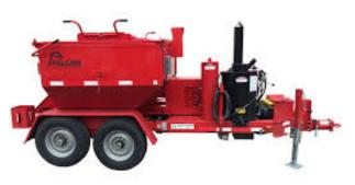
will also allow us to keep the mix at working temperatures for extended work times. The extended work time allows for doing patch work in high volume traffic areas overnight during off peak times. In the winter months, this unit will have the capacity to re-heat virgin hot mix asphalt that has been stockpiled from warmer months. The re-heated material is far superior to the winter cold patch commonly used.
